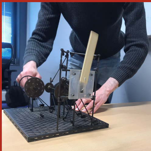
Figure 14: The Kapitza Pendulum in motion
